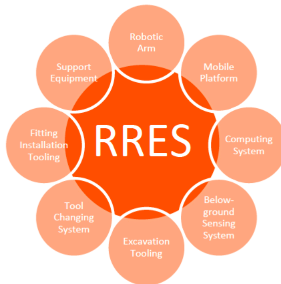
Figure 3: Simplified Systems Components
