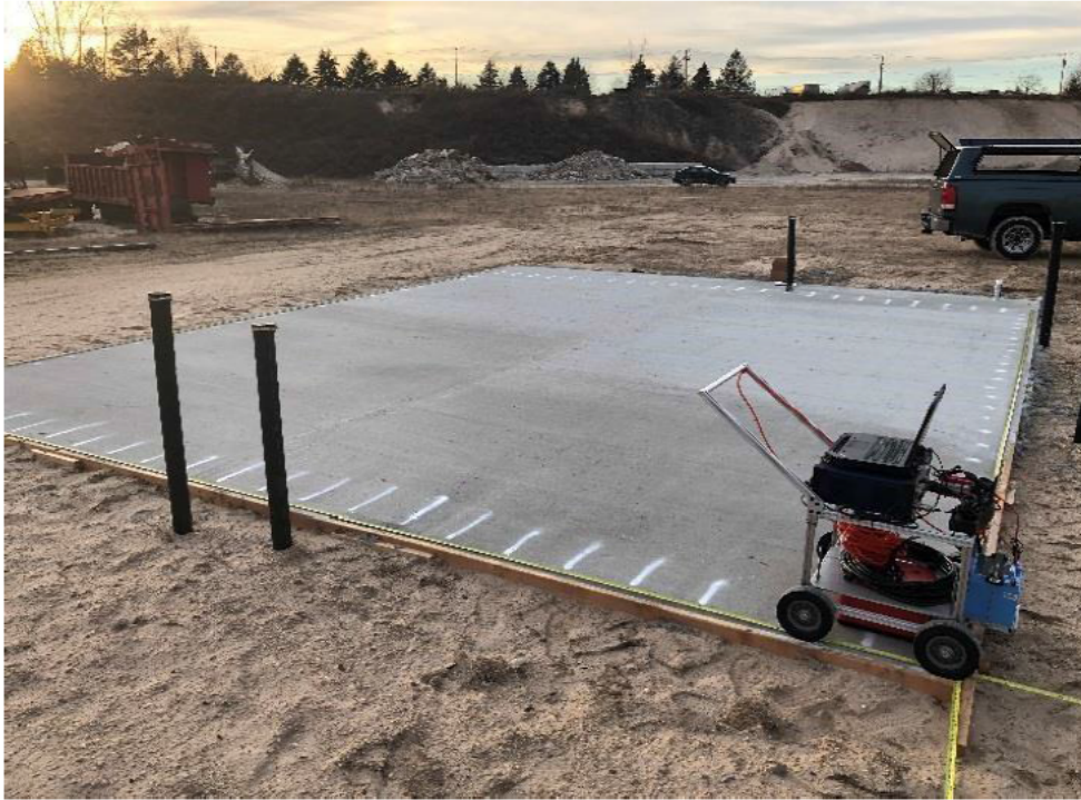
Figure 20 - Scanning the RRES mock roadway using the custom GPR system.
