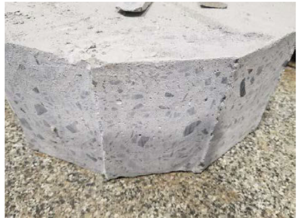
Figure 4 - 12" diameter plunge-only cut test
