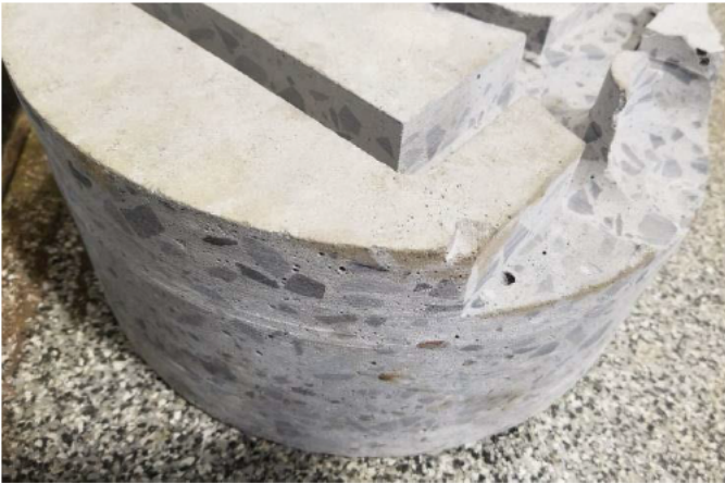
Figure 3 - Initial round cut performed slowly with a wide kerf chain
